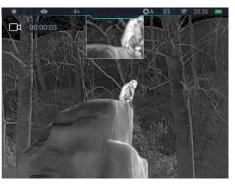
the image in the PIP window will also be enlarged by 2 times accordingly. For example, if the main image is enlarged by  $1\times$ ,  $2\times$ ,  $3\times$ , or  $4\times$ , the image in the PIP window will be enlarged by  $2\times$ ,  $4\times$ ,  $6\times$ , or  $8\times$ respectively.
